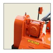
Gear Box with an input speed of 540 RPM.
