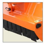
The front safety flaps made of steel allow material to enter the cutting frame but prevent inside objects from being expelled outside at high operating speed.
