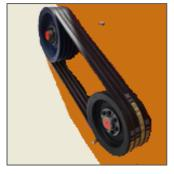
3 Belts & 4 belts (BX Type) transmission to transfer power to the rotor.
